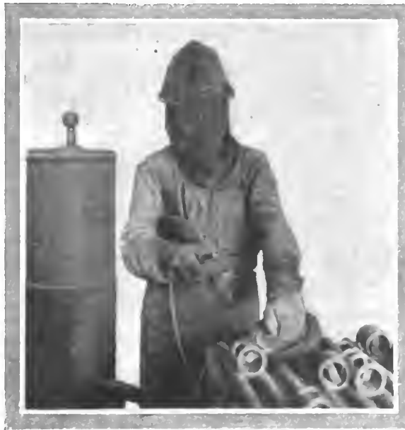
Workman In Garb and Mask Sanding Drop Forgings to Remove the Scale
